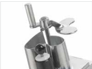
Integral safety inter-locks ensure safe product loading
